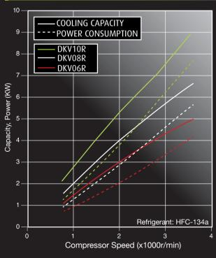
**TEST CONDITIONS** Discharge pressure: 1.52MPa (gage) Suction pressure : 0.18MPa (gage) Sub cool :5°C Super heat : 10°C
